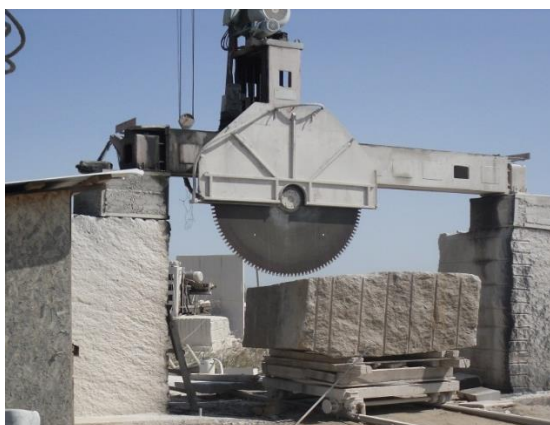
Fig. 1. The process of sawing a granite block with a circular diamond saw
